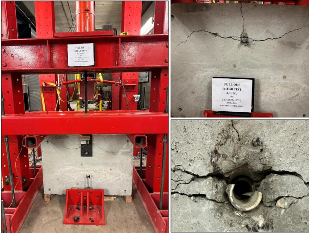
**Figure D1.1** The image of the specimen before failure and after failure.
