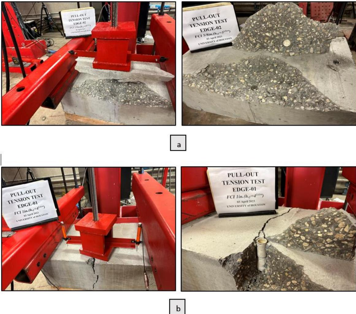
**Figure 25.** Failure mode (edge): **a)** concrete breakout cone failure and **b)** splitting failure.
