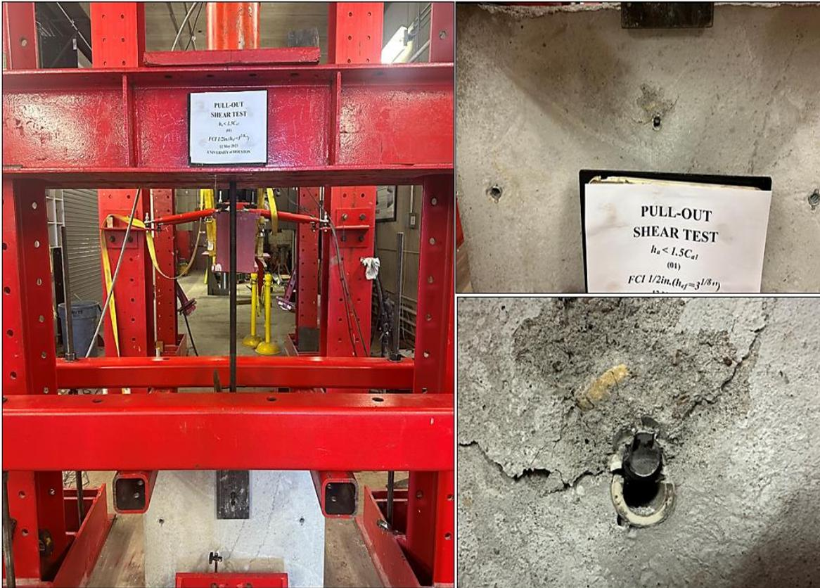
**Figure D5.1** The image of the specimen before failure and after failure.
