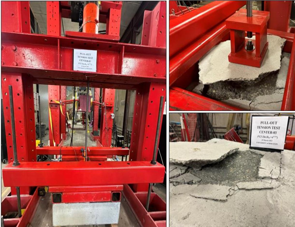
Figure A2.3 The image of the specimen before failure and after failure.
