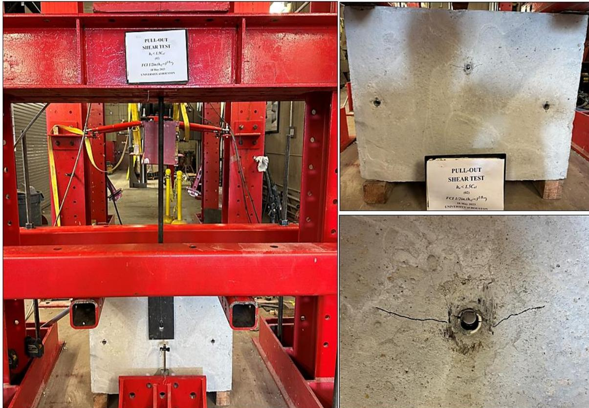
**Figure D5.2** The image of the specimen before failure and after failure.
