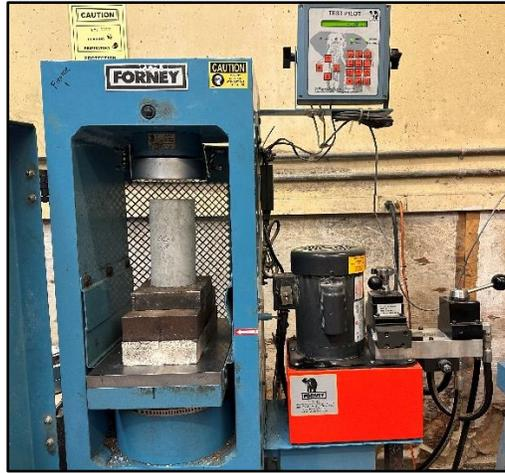
**Figure 12.** Setup of the compressive strength tests.
