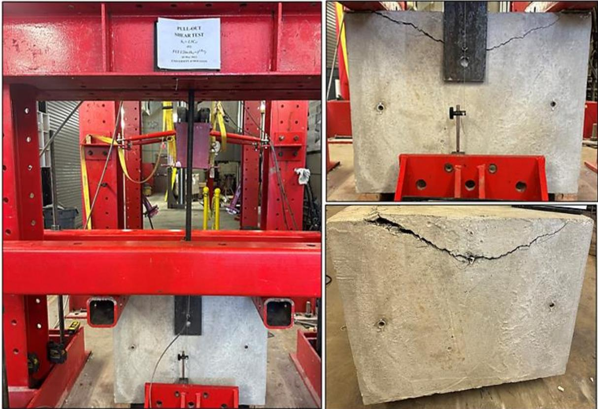
**Figure C5.2** The image of the specimen before failure and after failure.
