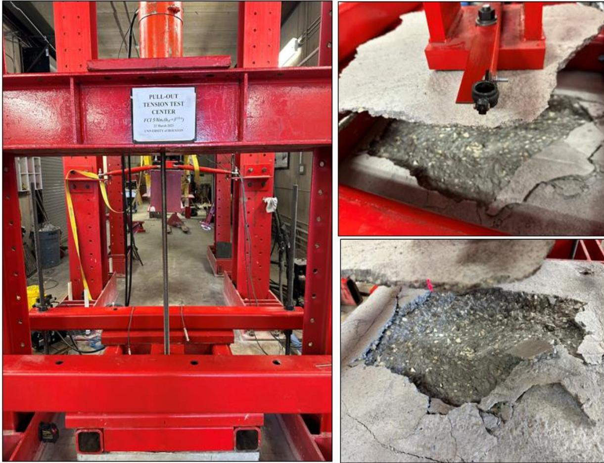
**Figure A3.1** The image of the specimen before failure and after failure.
