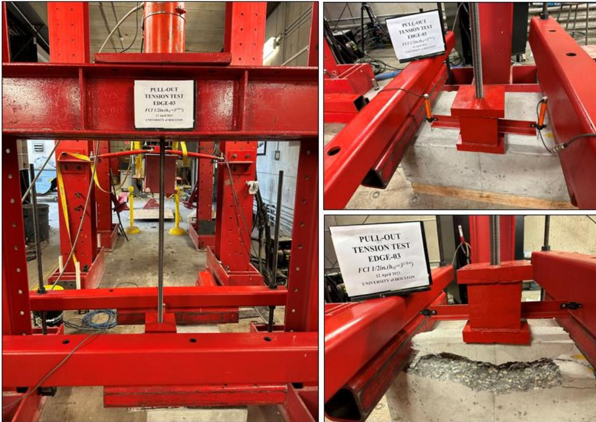
Figure B5.3 The image of the specimen before failure and after failure.
