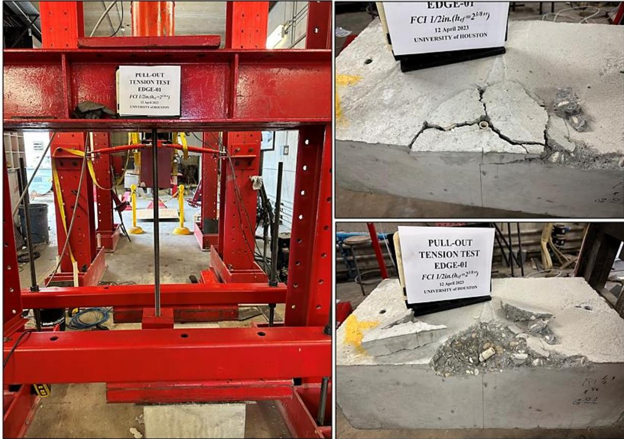
**Figure B6.1** The image of the specimen before failure and after failure.
