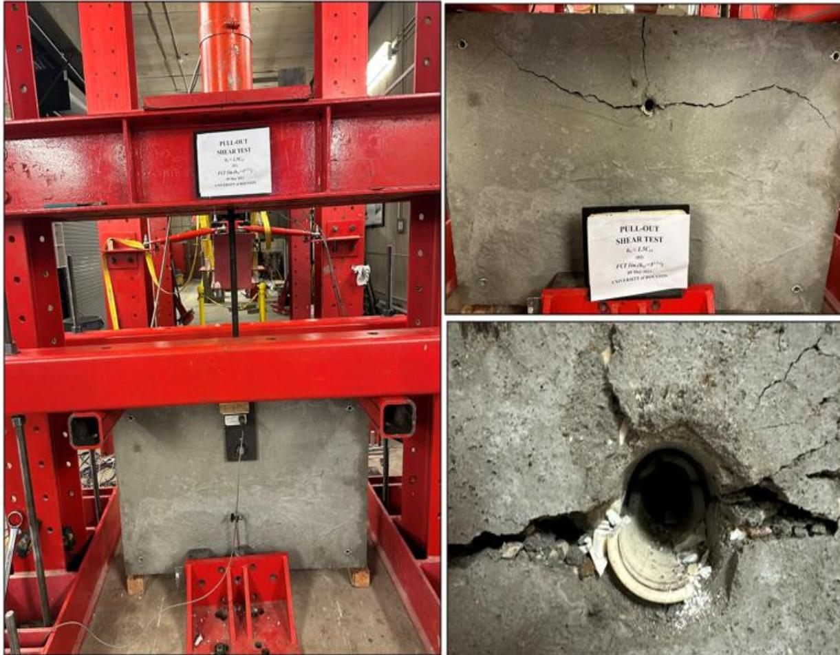
**Figure D1.2** The image of the specimen before failure and after failure.
