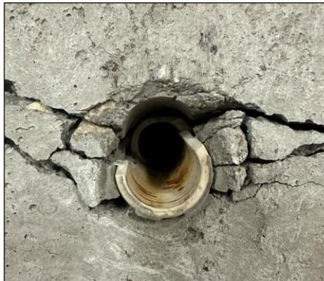
**Figure 37.** FCI insert fracture at the top.
