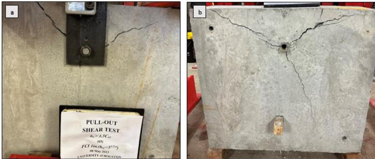
**Figure 27.** Failure mode for FCI 1in. ( $h_a > 1.5C_{a1}$ ): **a)** concrete breakout cone failure and **b)** vertical crack along the depth of the specimen.
