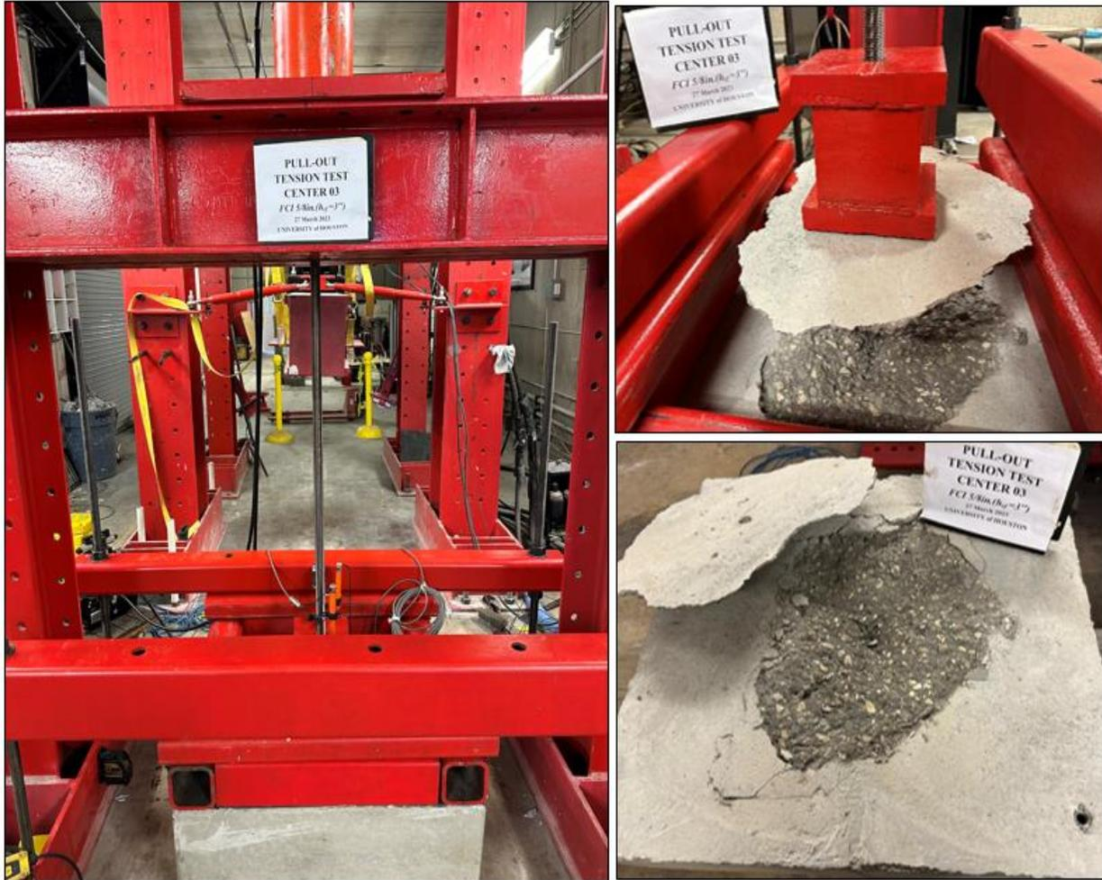
**Figure A4.3** The image of the specimen before failure and after failure.
