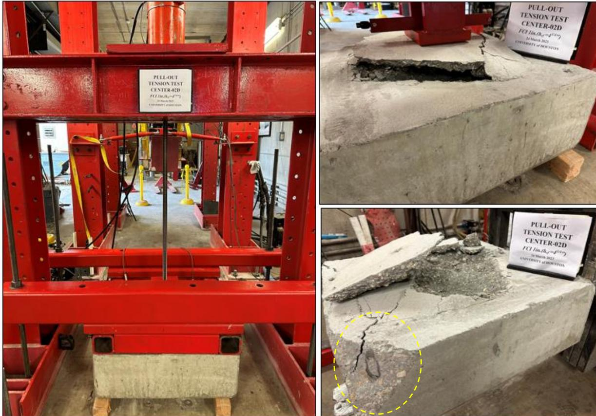
Figure A2.2 The image of the specimen before failure and after failure.
