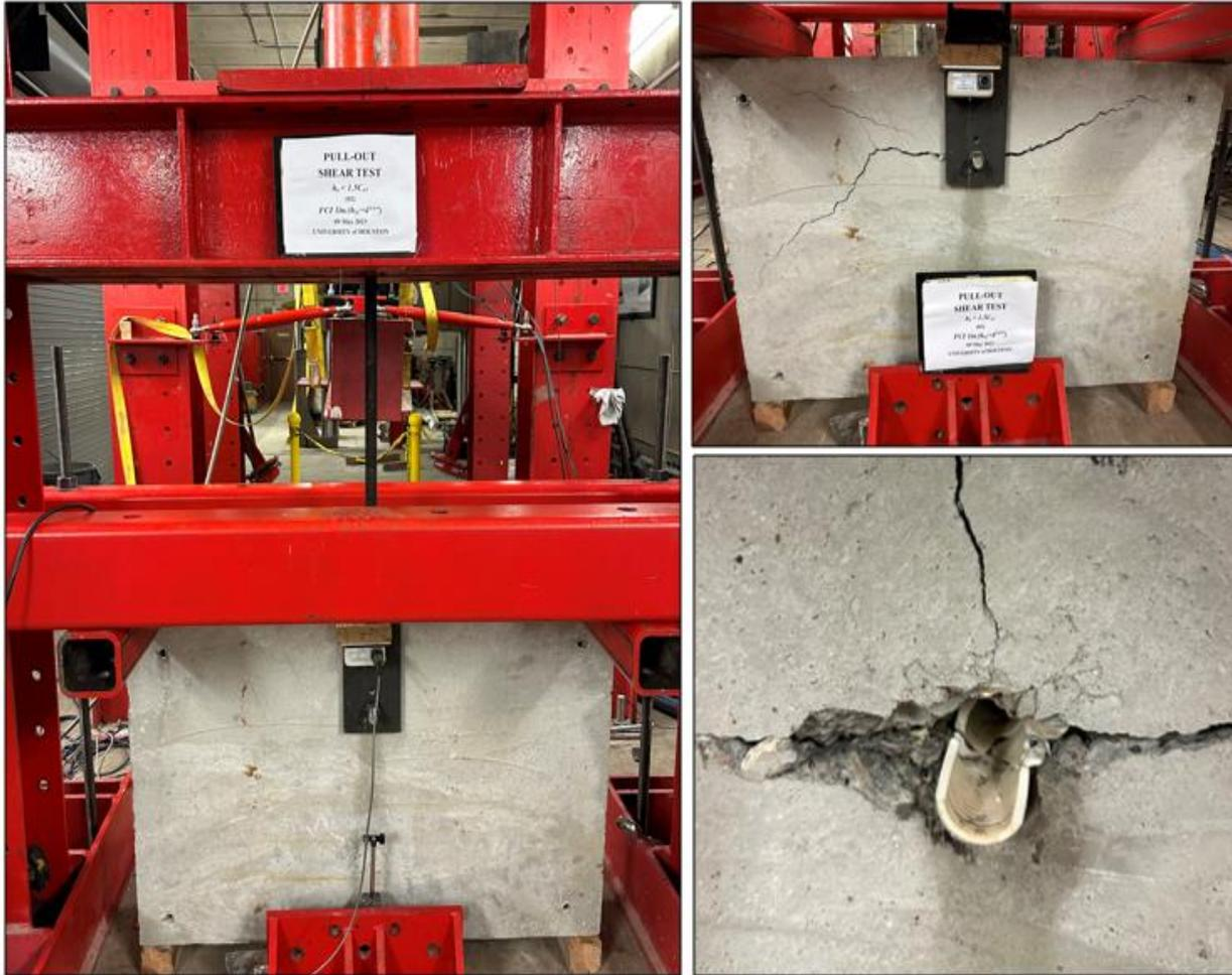
**Figure D2.2** The image of the specimen before failure and after failure.
