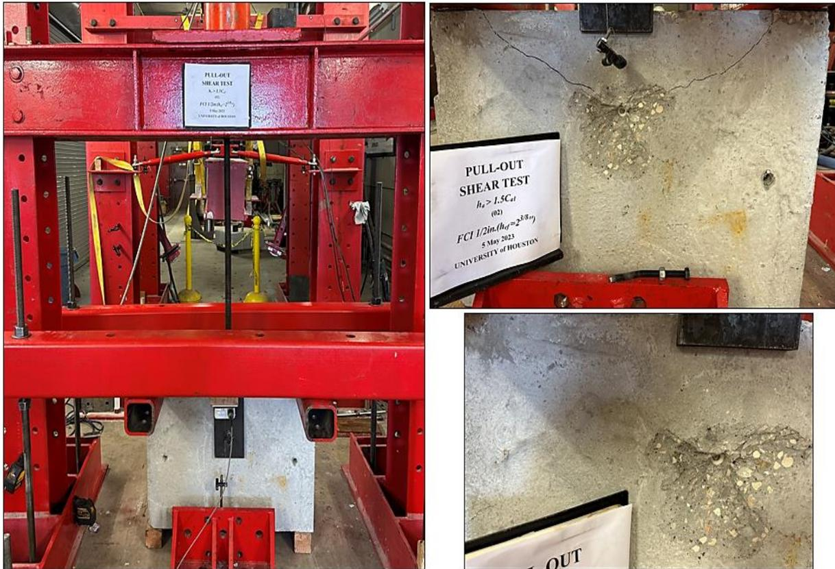
**Figure D6.2** The image of the specimen before failure and after failure.
