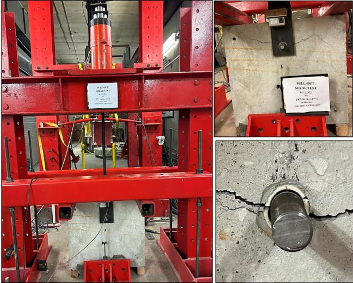
Figure C2.3 The image of the specimen before failure and after failure.
