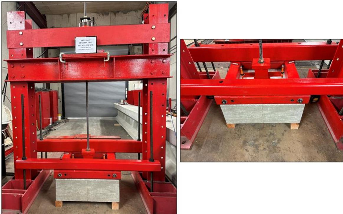
**Figure 15.** Experimental setup for the tension test.
