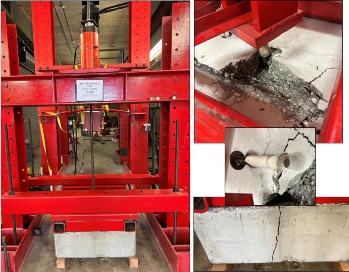
**Figure A1.1** The image of the specimen before failure and after failure.
