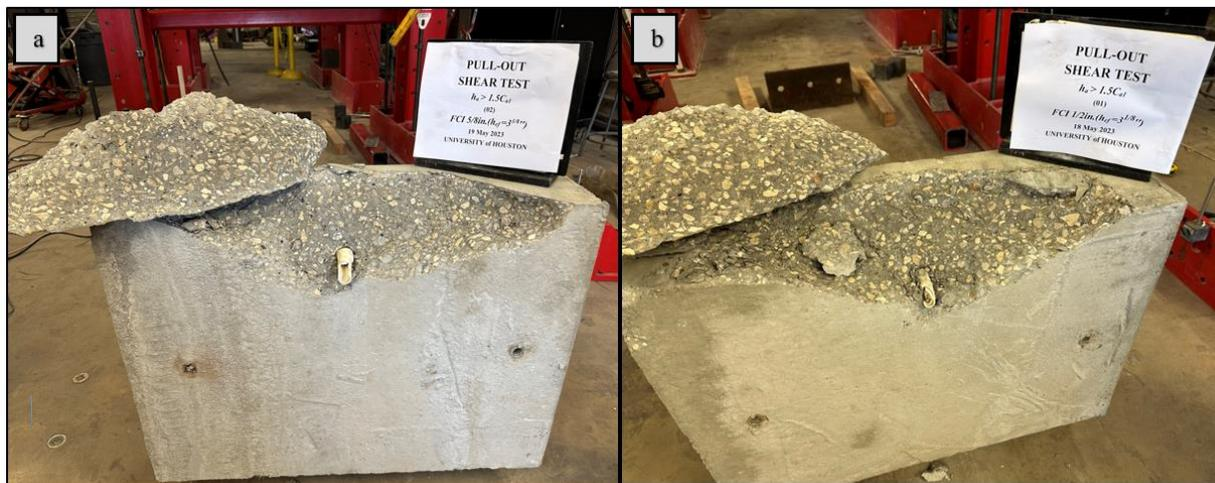
**Figure 31.** Failure mode of (a) FCI 5/8in. and (b) FCI 1/2in.
