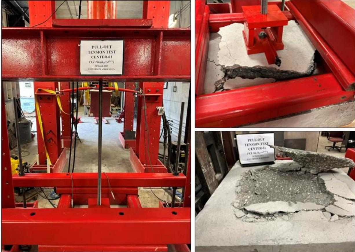
**Figure A2.1** The image of the specimen before failure and after failure.
