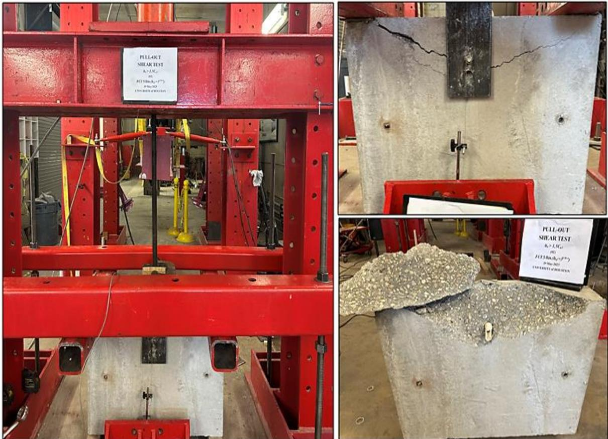
Figure C3.2 The image of the specimen before failure and after failure.
