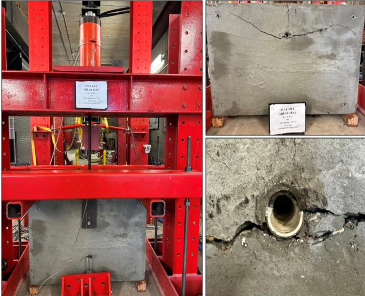
**Figure D1.3** The image of the specimen before failure and after failure.
