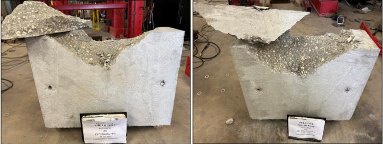
**Figure 34.** Failure mode for FCI 5/8in. ( $h_d < 1.5C_{at}$ ): concrete breakout cone failure.
