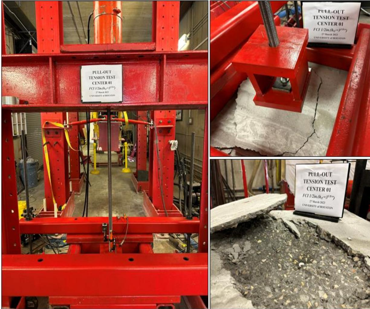
Figure A5.1 The image of the specimen before failure and after failure.
