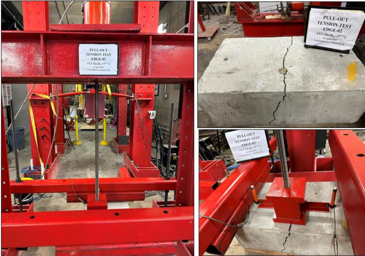
**Figure B1.2** The image of the specimen before failure and after failure.
