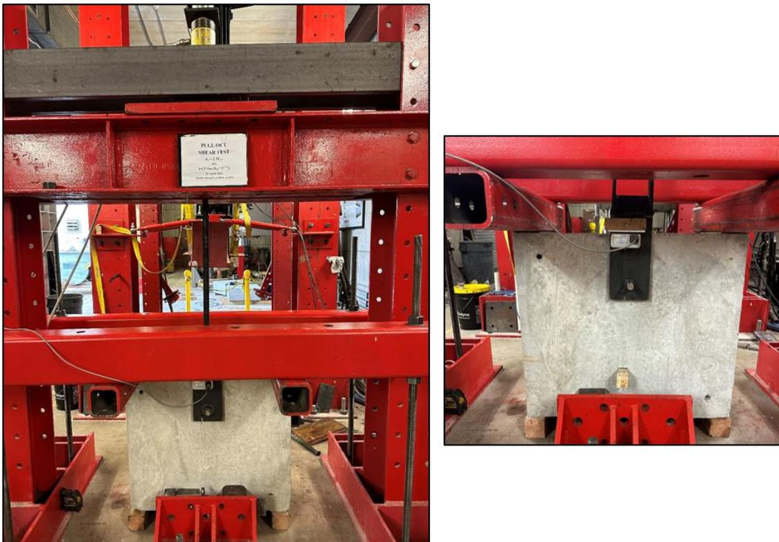
**Figure 19.** Experimental setup for the shear test.
