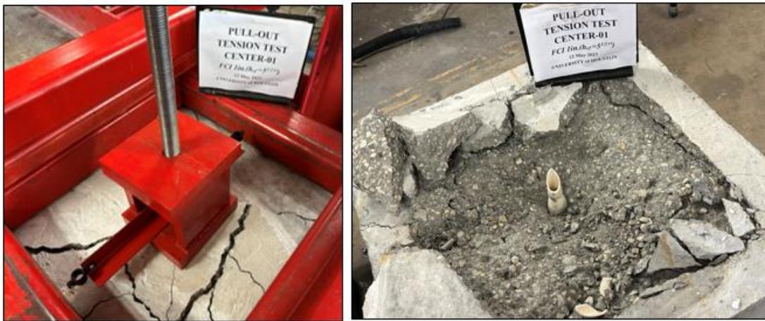
**Figure 23.** Failure mode of the FCI 1in. (center) with specimen thickness  $3 h_{ef}$ .
