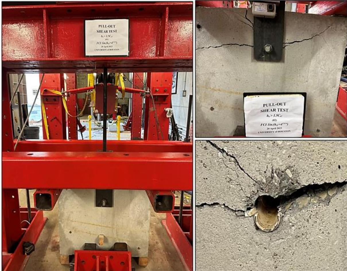
Figure C2.2 The image of the specimen before failure and after failure.
