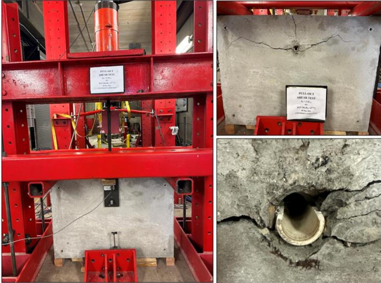
**Figure D2.1** The image of the specimen before failure and after failure.
