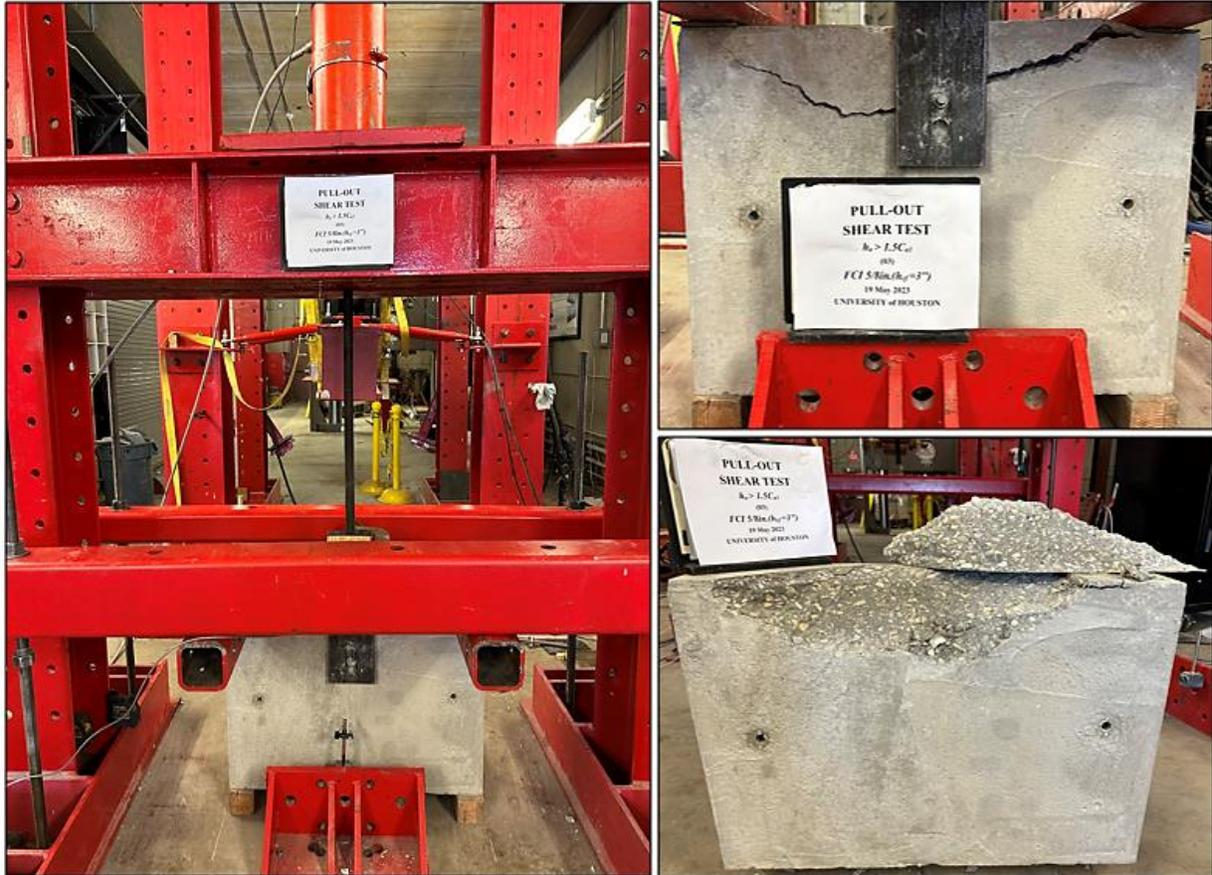
Figure C4.3 The image of the specimen before failure and after failure.
