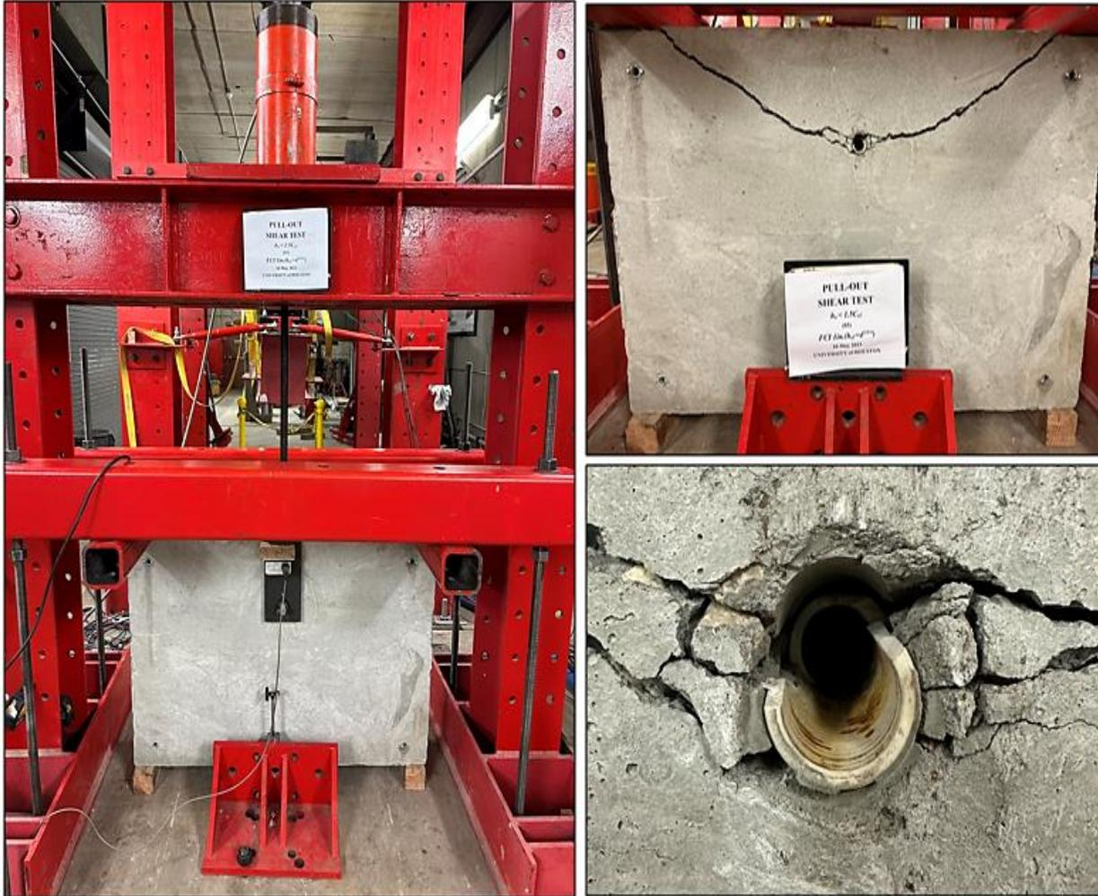
Figure D2.3 The image of the specimen before failure and after failure.
