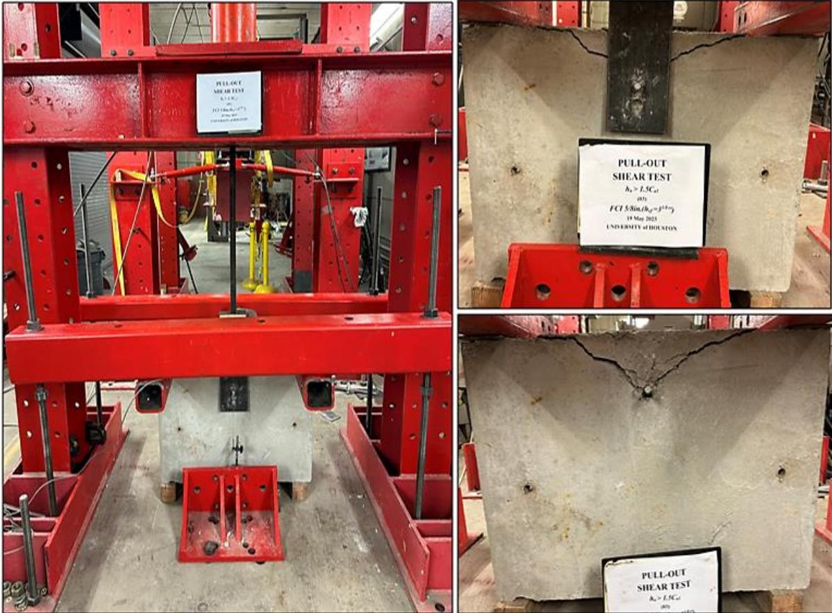
Figure C3.3 The image of the specimen before failure and after failure.
