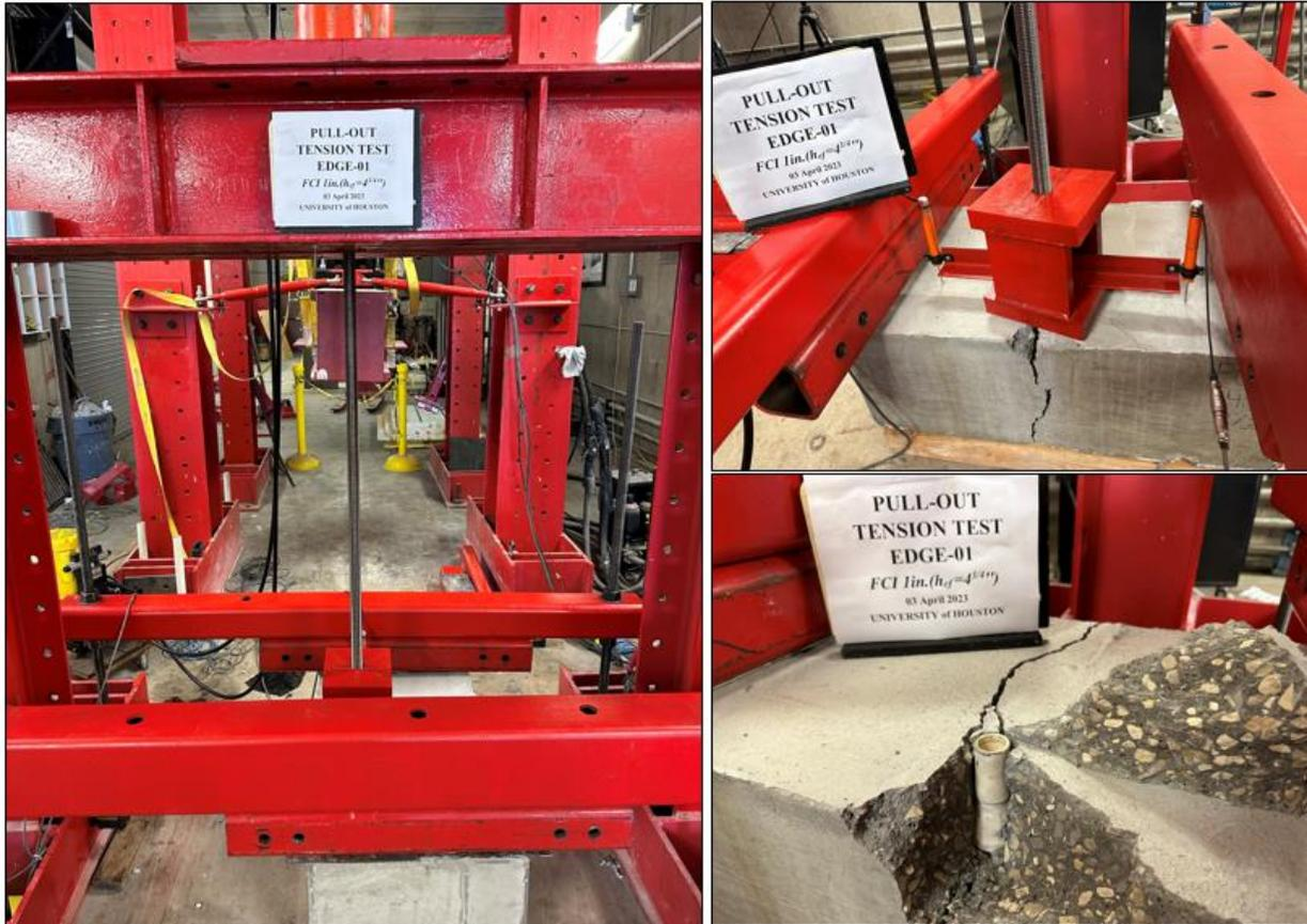
**Figure B2.1** The image of the specimen before failure and after failure.
