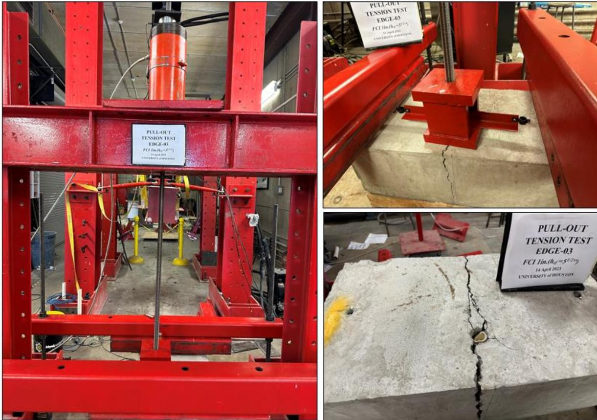
**Figure B1.3** The image of the specimen before failure and after failure.
