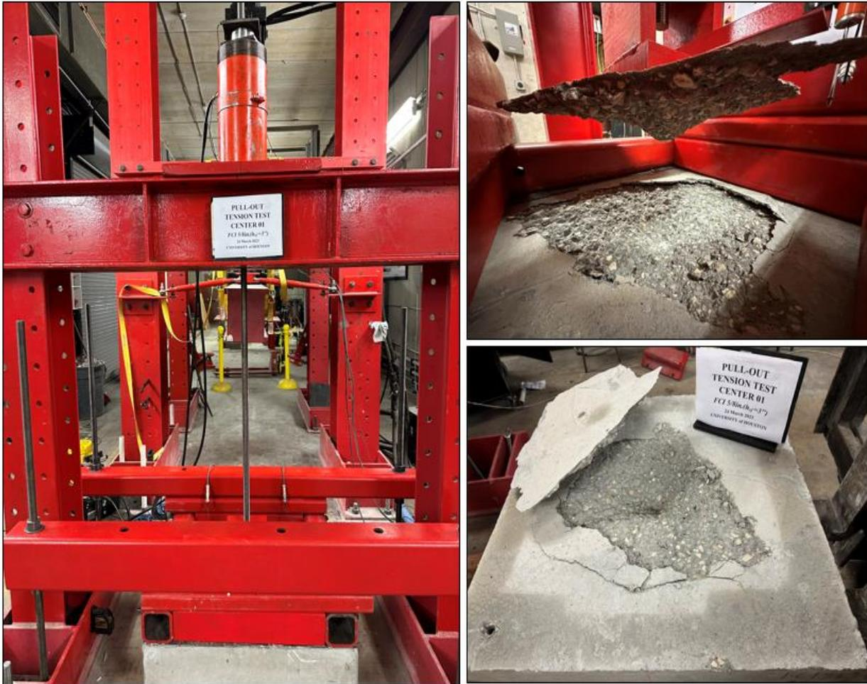
**Figure A4.1** The image of the specimen before failure and after failure.
