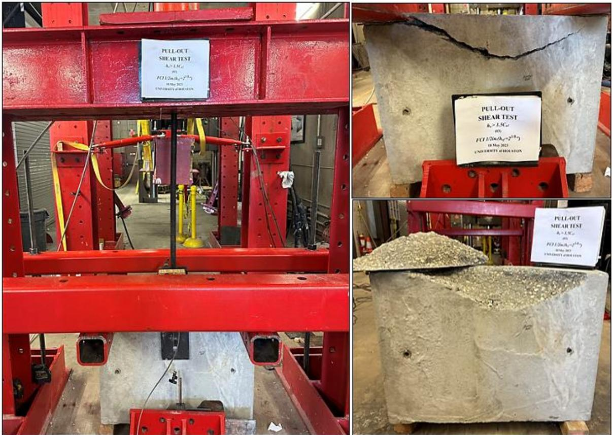
Figure C6.3 The image of the specimen before failure and after failure.
