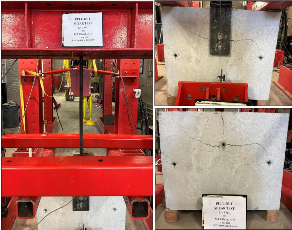
**Figure D4.2** The image of the specimen before failure and after failure.
