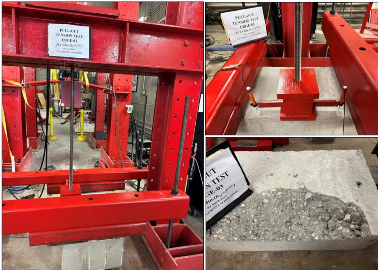
**Figure B3.3** The image of the specimen before failure and after failure.
