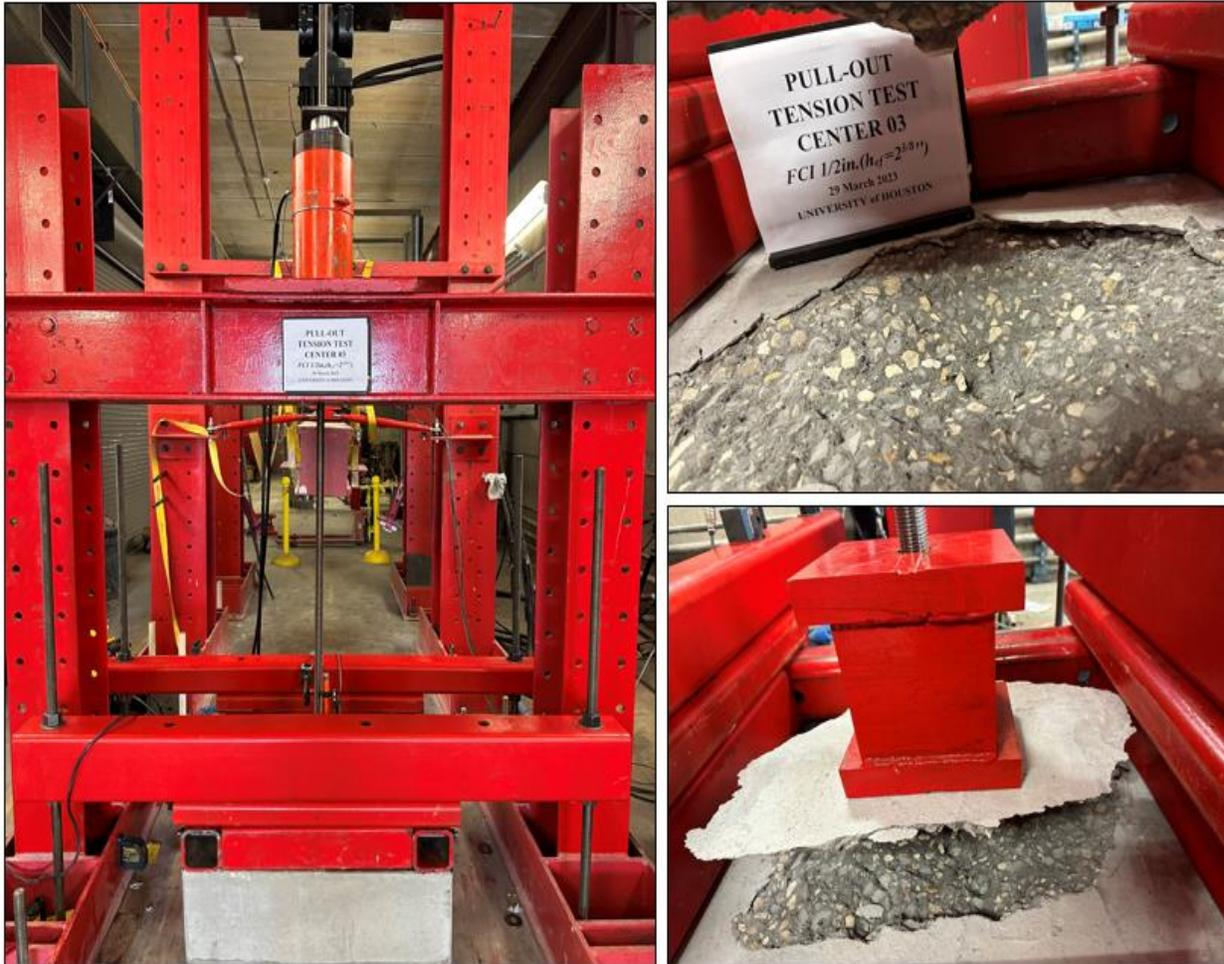
**Figure A6.3** The image of the specimen before failure and after failure.
