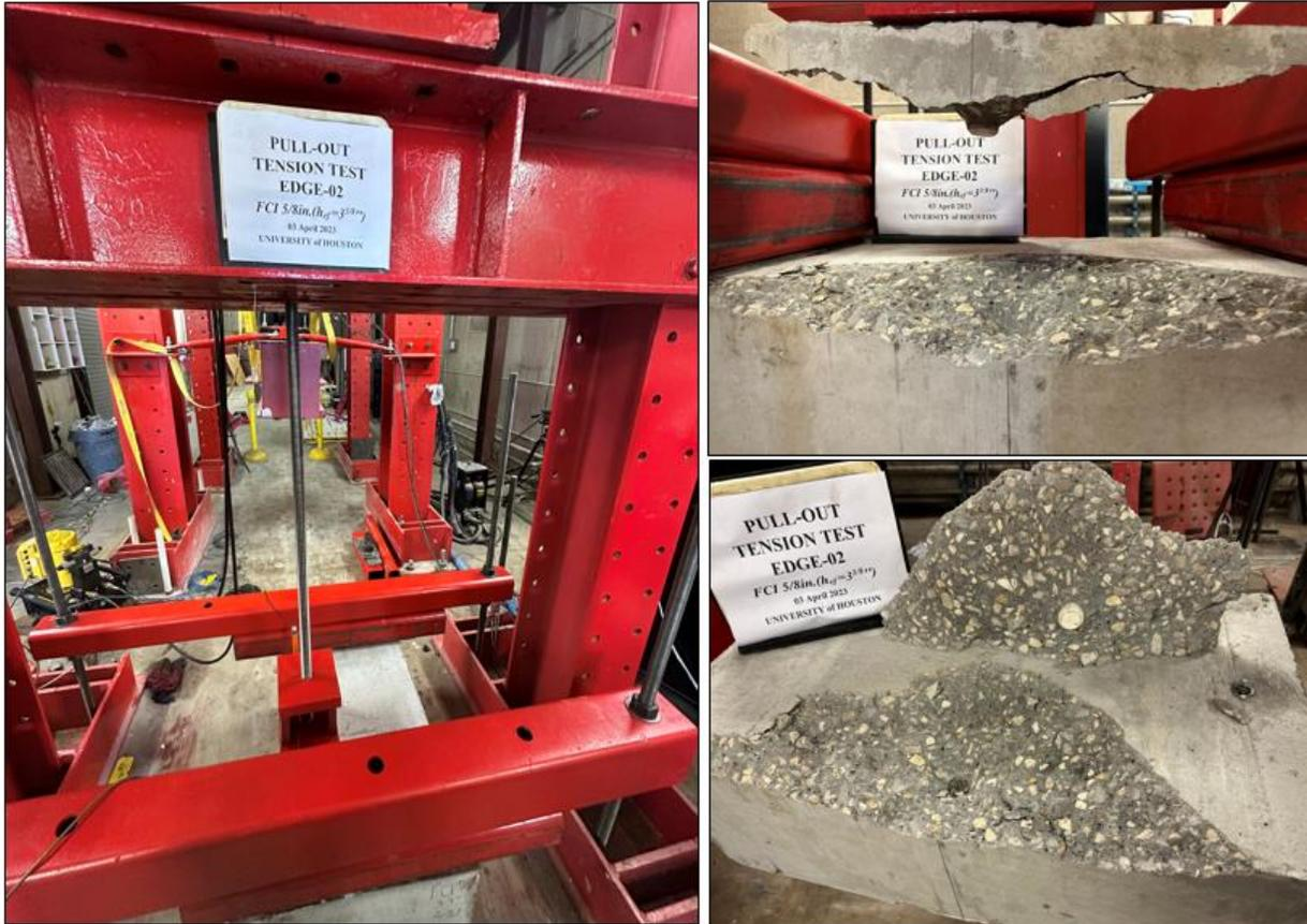
**Figure B3.2** The image of the specimen before failure and after failure.
