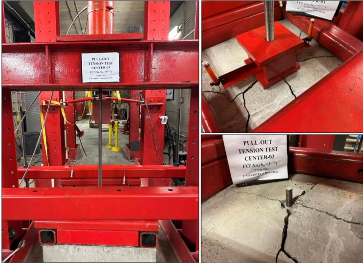
Figure A7.3 The image of the specimen before failure and after failure.
